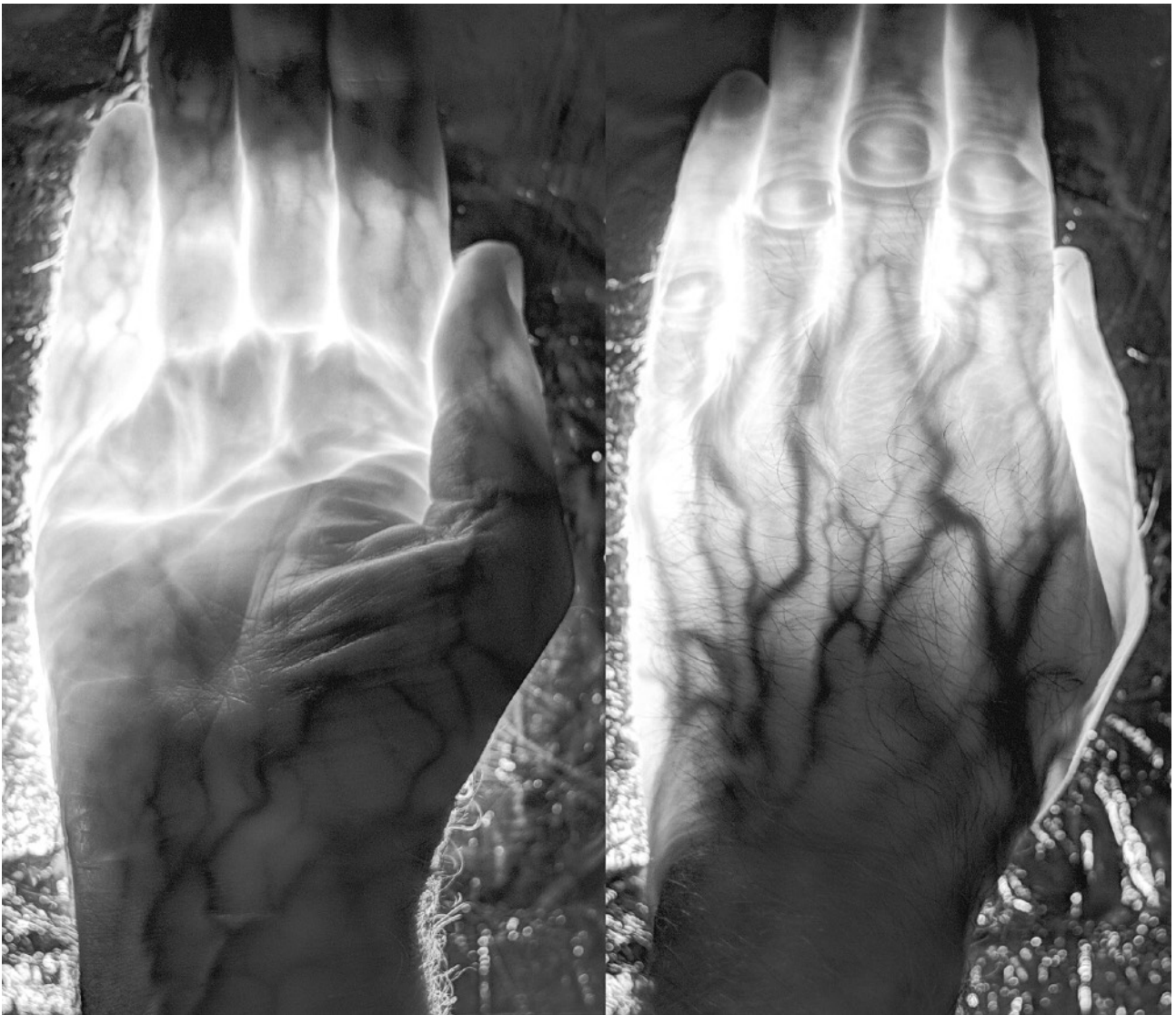
Figure 5. Images of a hand/wrist with palm up and down taken with a NIR (750 – 1,000nm) camera. The back illumination is from nine 850nm LEDs shining along a 140mm tube capped by an Al foil mask to avoid light leakage around the hand. Note that the veins are seen only where they are close to the upper skin surface, notably on the back of the hand on the right, but also on the wrist of the palm-up hand on the left. The bones are not seen. The tissue and bones act as an efficient light diffuser at this wavelength and the strongest (but still weak) absorber is the de-oxygenated blood in the veins: see Figure 6 where the spectrum is obtained from the region just below the thumb: the thickest part of the hand. These are high dynamic range images from multiple exposures combined with Photomatix Pro software.
