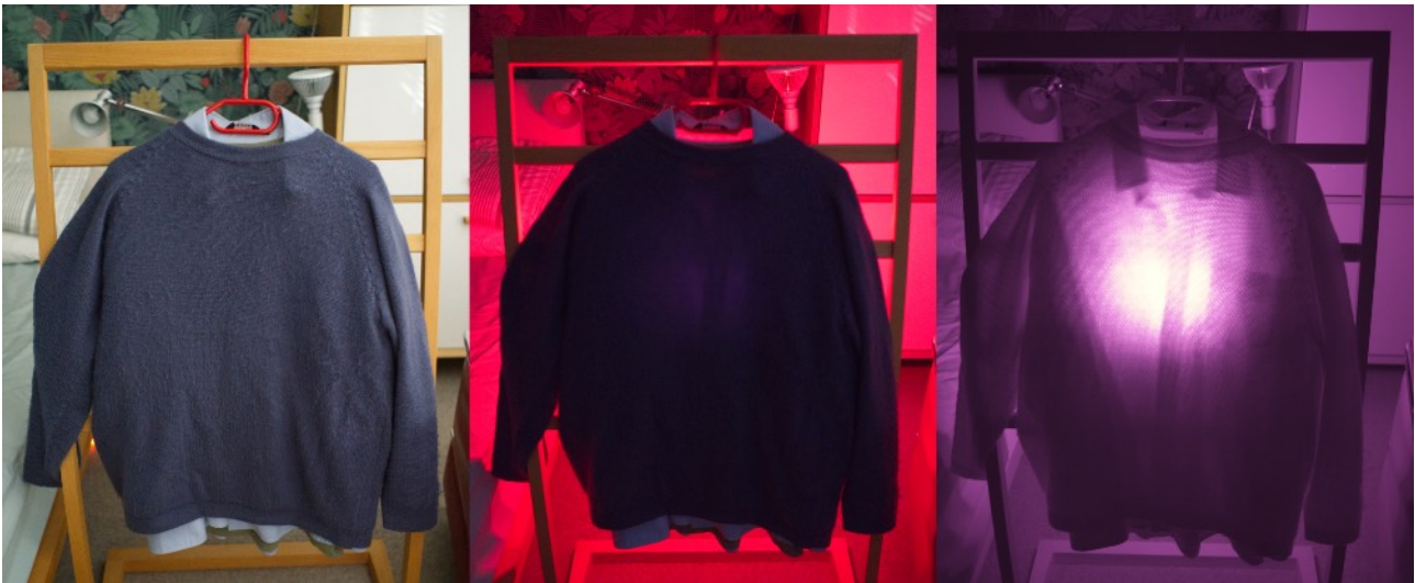
Figure 7. Do you need to remove your clothes to access NIR radiation? A T-shirt, a shirt and a woollen jumper on a hanger. Left: colour image in ambient daylight; Middle: colour image backlit with with an LED lamp emitting red (660nm) and NIR (850nm) light; Right: the same as the middle image but taken with an infrared (750–1000nm) camera. This shows that the clothes (six layers in all) are nearly 100 times more transparent at 850nm than at 660nm. The answer is the NIR light penetrates normal indoor clothing quite effectively.
